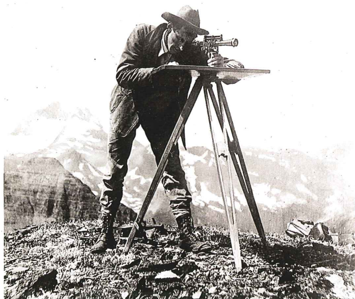
Figure 1. Herbert “Shortie” Clark mapping with a plane table and telescopic alidade in the early 1900s.
